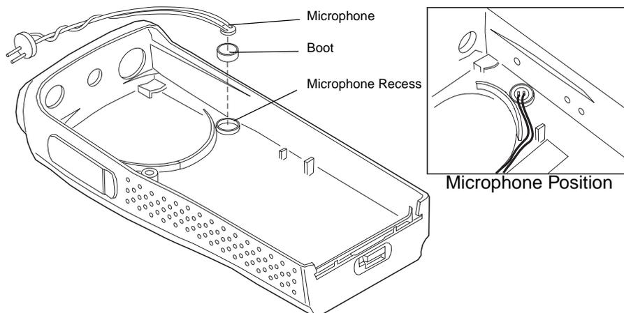
*Figure 8-10. Microphone Re-assembly*
