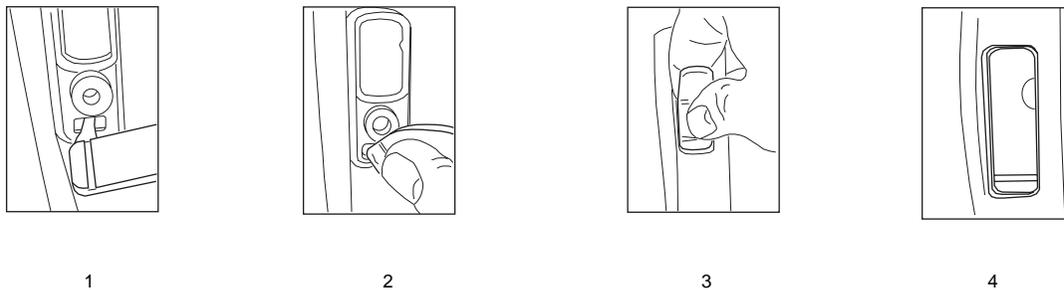
*Figure 6-11. Dust Cap Re-assembly*
