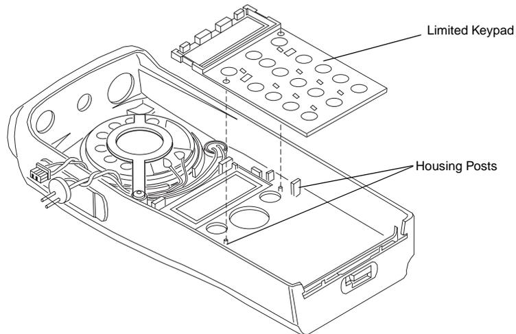
*Figure 7-14. Keypad Re-assembly*
