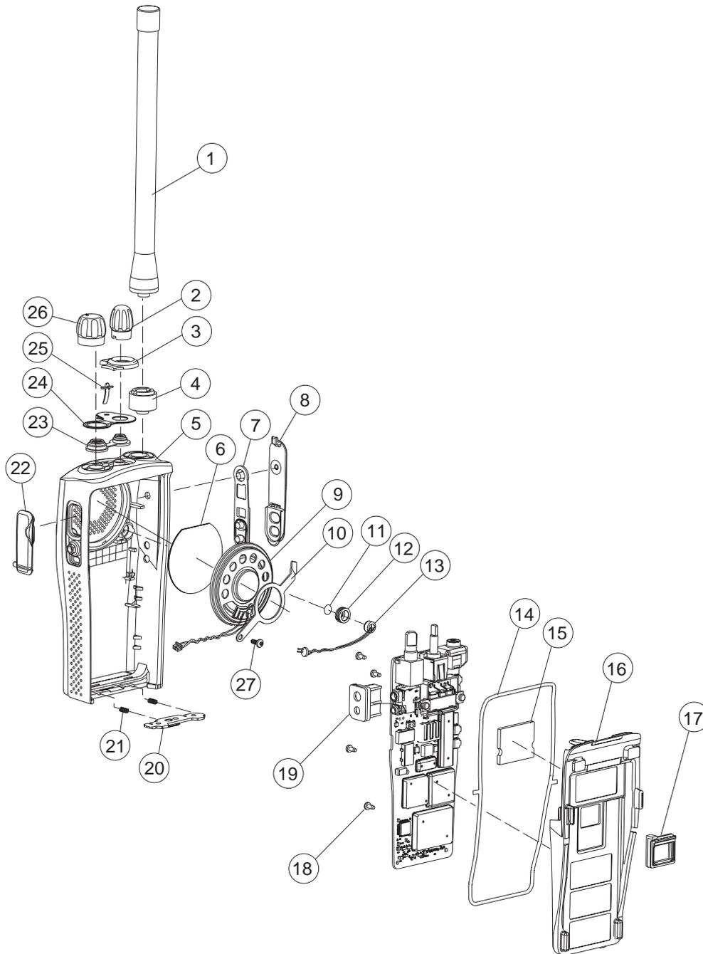
Figure 8-16. PR400 Non-Keypad Radio Exploded View
