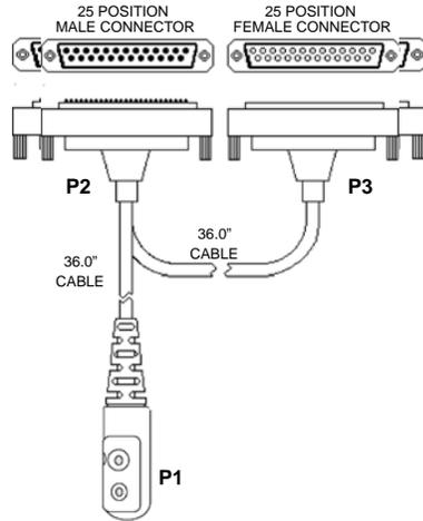
Figure 3-1. Programming/Test Cable
